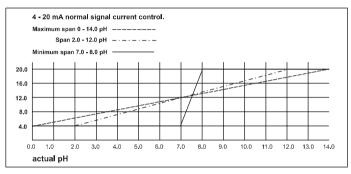
FIG 9 4-20mA normal Signal current control.
