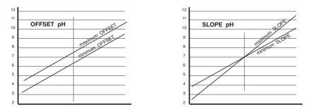
FIG. 6 THE DIFFERENT EFFECTS OF OFFSET AND SLOPE.
