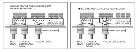
FIG 4 Wiring examples for the relay outputs.
