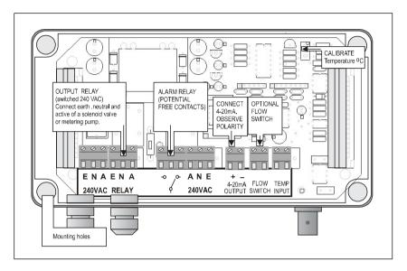
FIG 5 Terminal layout of the PPH-1.
