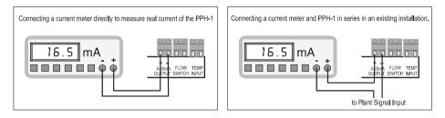
FIG 11 4-20mA Setpoint Signal current control.
