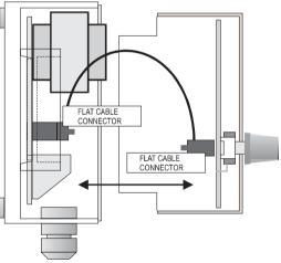
FIG 3 CHASSIS & removable FACIA of the PPH-1
